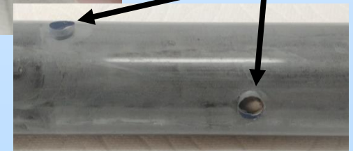
Perforations in support pipe enable liquid permeation
