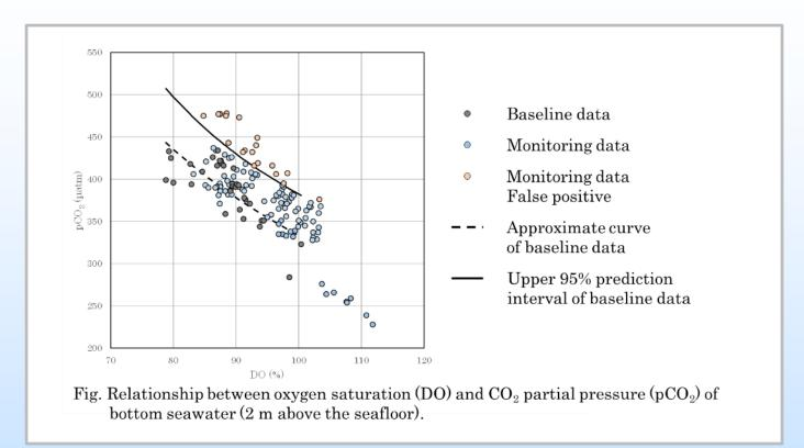
"Regulatory authority urged strongly to use the relationship between concentrations of oxygen and carbon dioxide to detect leakage. Since the baseline data did not fully reflect the natural variation, false positive occurred. Ultimately, the observed value (false positives) were judged to be within the range or natural variation by the expert judge. In other words, no leakage was observed".
