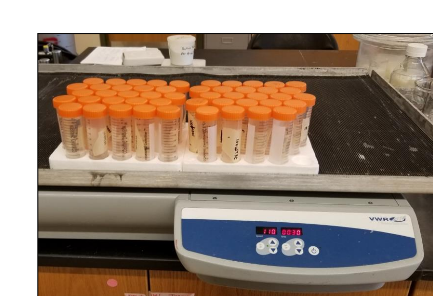
Figure 3: Analyzing Salt solutions of various concentration at different times in the Shake Table
