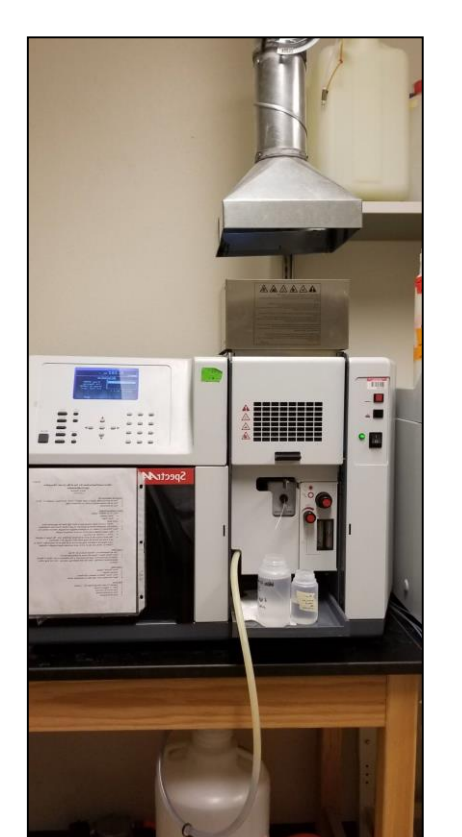
Figure 4: Use of Atomic absorption spectrometry to determine the concentration of Cations
