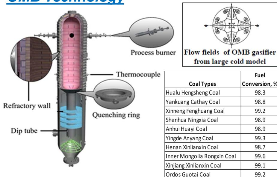
oResidence time independent of the gasifier size oEspecially suitable for small-scale modular application oScale-up demonstrated but small scale modular study needed
