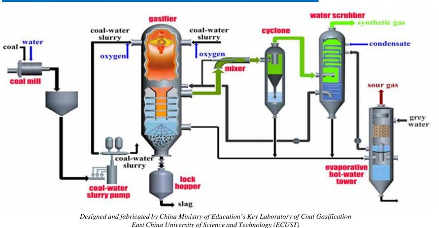
oGasification, quench chamber and water scrubber oDry coal consumption: 1 ton/day oH/CO: ~0.75/1
