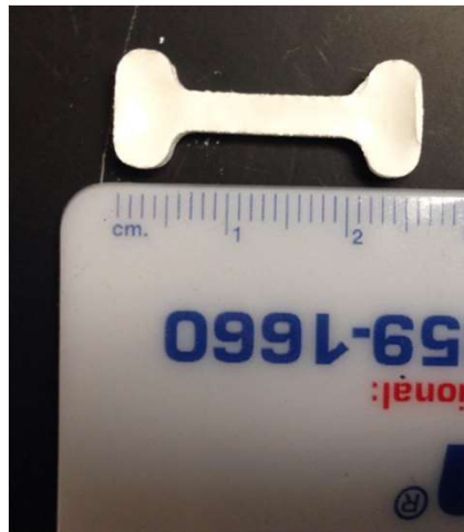
Dog-bone shaped sample from slip casting
