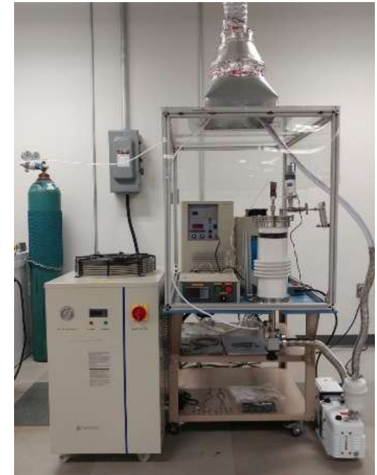
2000°C Temperature-Controlled 30KW Induction Heating System (MTI Corp., EQ-SP-50KTC)
