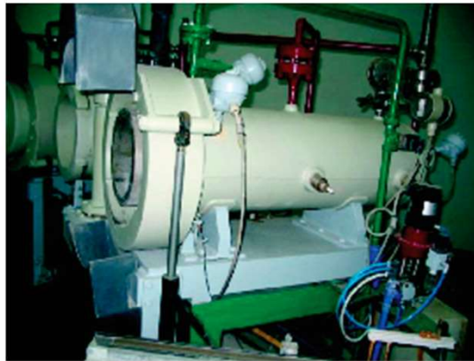
SHS reactor for industrial production of powders.
