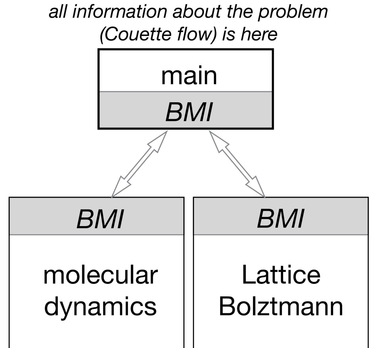
*The BMI handles all communication with the models: input, instructions, output, ... through a standard set of functions.*
