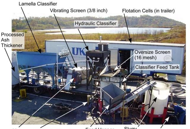
Vacuum Hydraulic Classifier Filter Feed Pump
