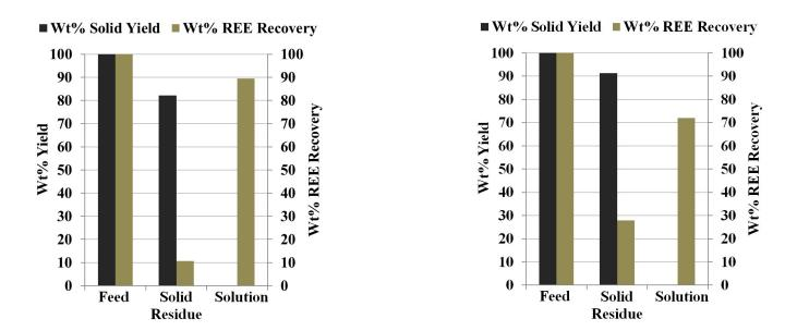
Solid Residue Yield and REE Recovery to Solution, Samples A and B, 700 by 100 micron fraction, 1 hour in Ammonium Sulfate Solution
