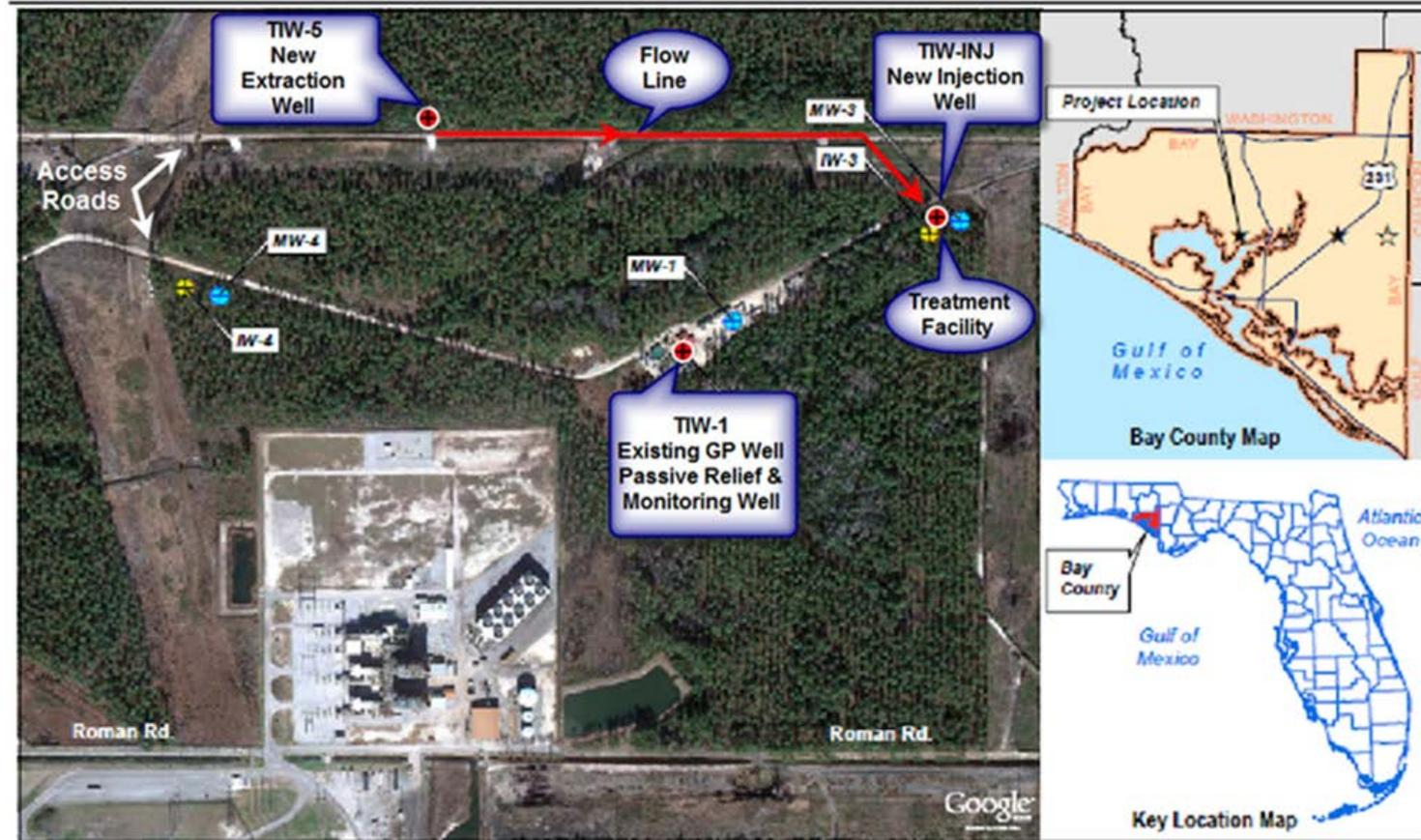
BEST project infrastructure layout showing the proposed location of the extraction well (TEMW-A), injection well (TIW-2) and flowline, and the existing passive-relief well (TIW-1)
