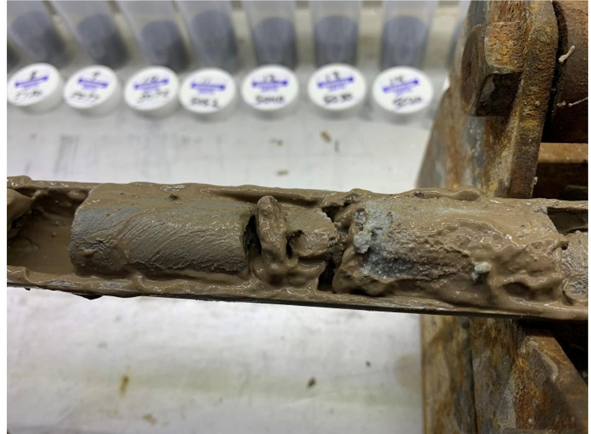
Close-up view of side-wall cores
