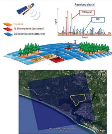
**Joint Inversion** - We will use LBNL's powerful inverse modeling and parameter estimation tool iTOUGH (in its parallel version MPiTOUGH2) for the automated joint inversion of hydrological, large-scale geophysical (EM) data, and surface deformation data.
