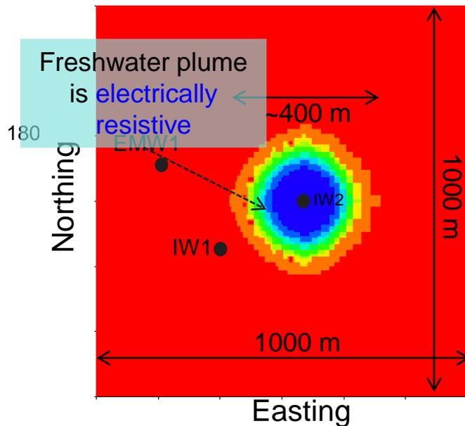
Surface-to-borehole EM configuration with proposed transmitter locations
