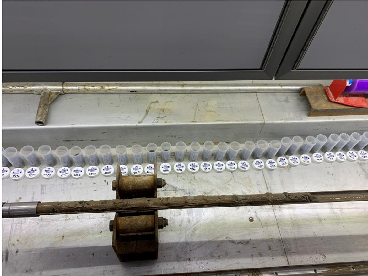
Core barrel containing continuous side-wall cores
