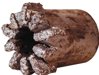
The Drag Bit is the most commonly used drill bit for marine soil investigations.
