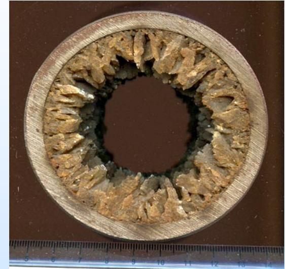
Barite deposition in casing (pipe) during production. *From Stack, <https://www.epa.gov/sites/products/files/documents/stack.pdf>*
