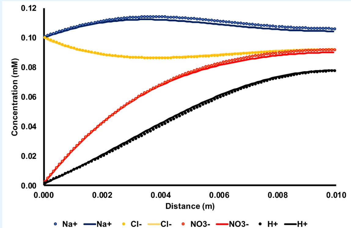
2. Tracer isotope ( $^{22}\text{Na}^+$  vs  $\text{Na}^+$ ) diffusion due to charge effects<sup>1</sup>. PHREEQC (symbols), **Osures** (solid) steady-state  $^{22}\text{Na}^+$  concentration
