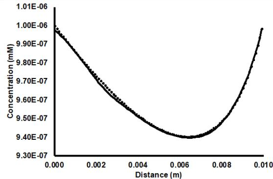
2. Tracer isotope ( $^{22}\text{Na}^+$  vs  $\text{Na}^+$ ) diffusion due to charge effects<sup>1</sup> PHREEQC (symbols), **Osures** (solid) steady-state  $^{22}\text{Na}^+$  concentration
