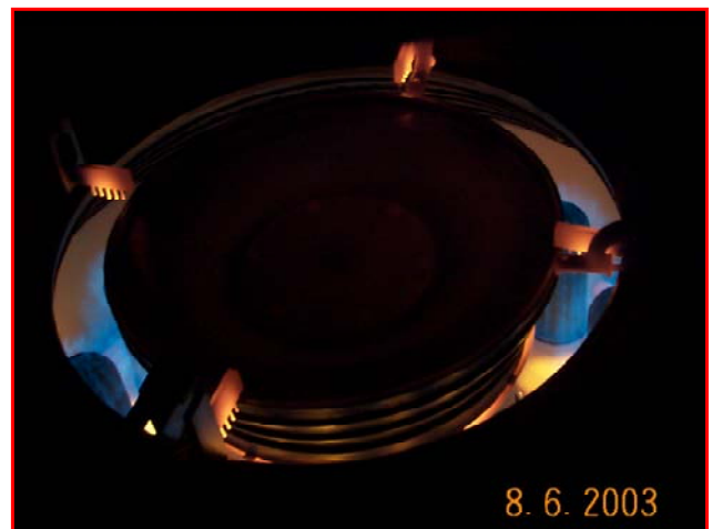
Fig. 6. Interior of Full Scale Annular Combustor during Atmospheric Testing (reproduced by permission of the publisher from American Society of Mechanical Engineers [ASME]).
