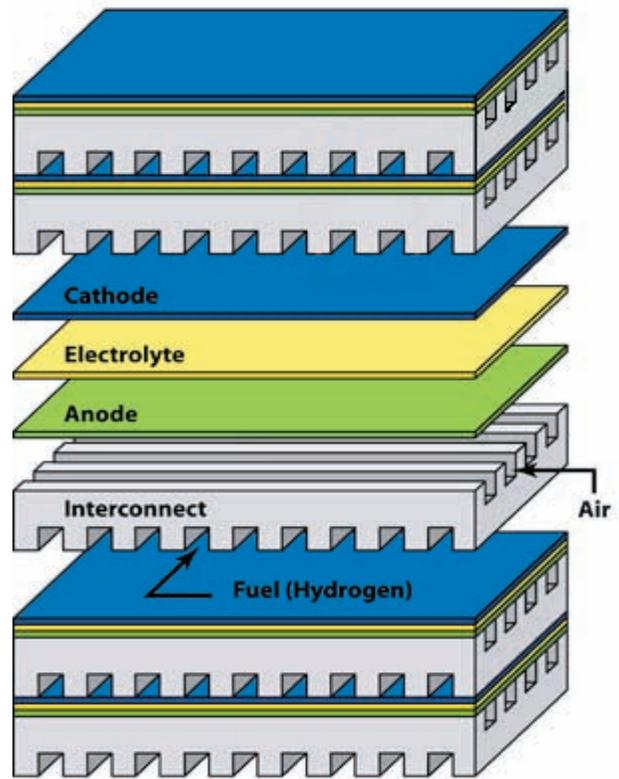
Fig. 2. Basic components of a fuel cell stack
