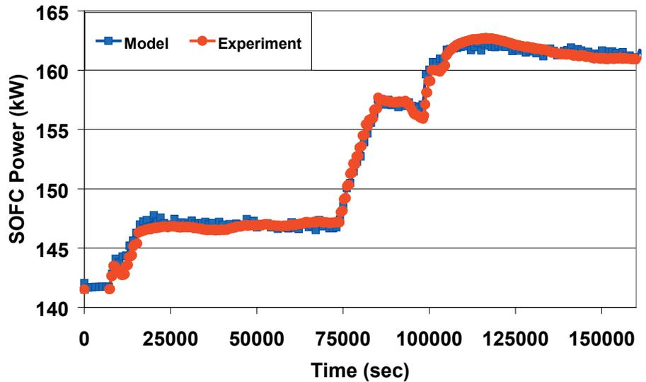
Fig. 12. SOFC power experimental and simulation comparison
