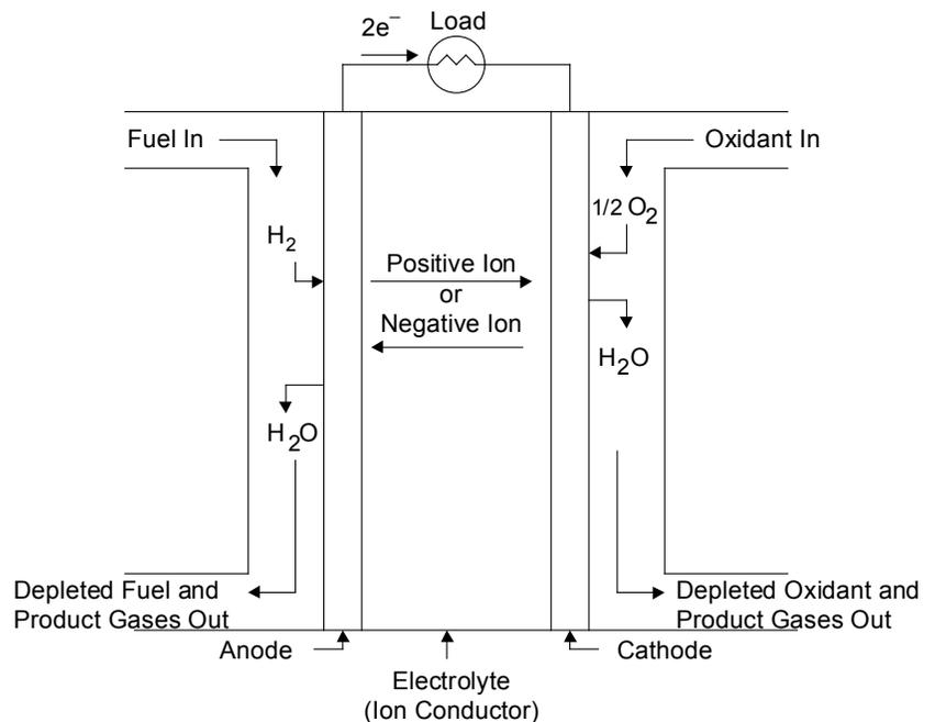
Fig. 1. General schematic of a fuel cell
