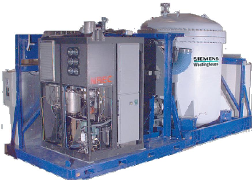
Fig. 7. Pressurized 220 kW SOFC/Gas Turbine Hybrid
