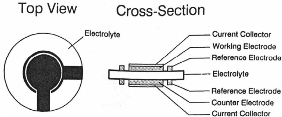
Porous Nanocomposite Electrode
