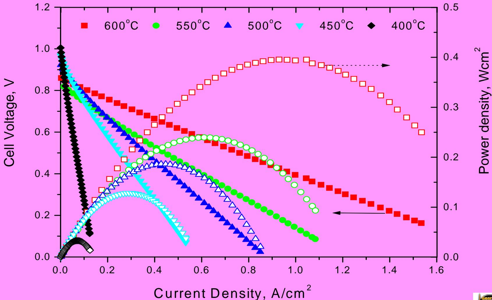
Fuel: humidified (3 v% H<sub>2</sub>O) hydrogen; oxidant: air
