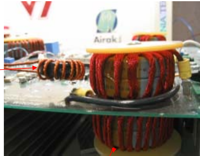
L_f for full-bridge converter
