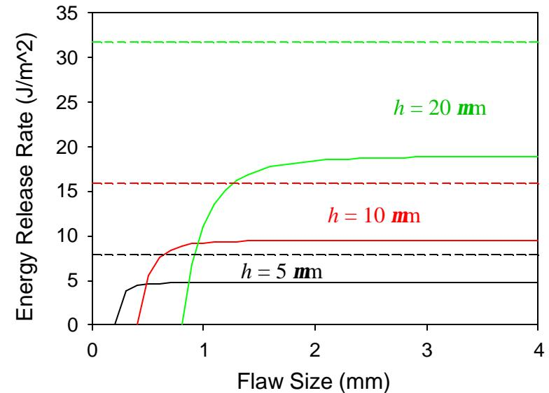
Comparison of energy release rate between edge and blister delamination
