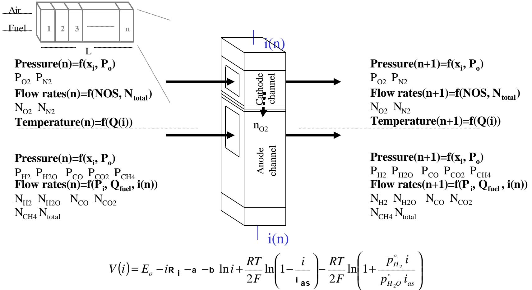
Electrochemical model is a combination of the polarization model of Kim et al. (1999) and Haynes' slice technique (Haynes and Wepfer, 1999)
