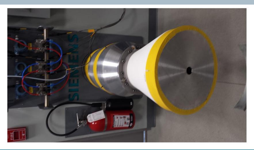
Full scale component assembly (attachments & seals) leakage testing conducted. Performance as expected based on coupon testing.
