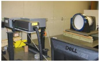
FTT shaker table used to validate modal analysis method. Apply validated method for CEC testing of cones.
