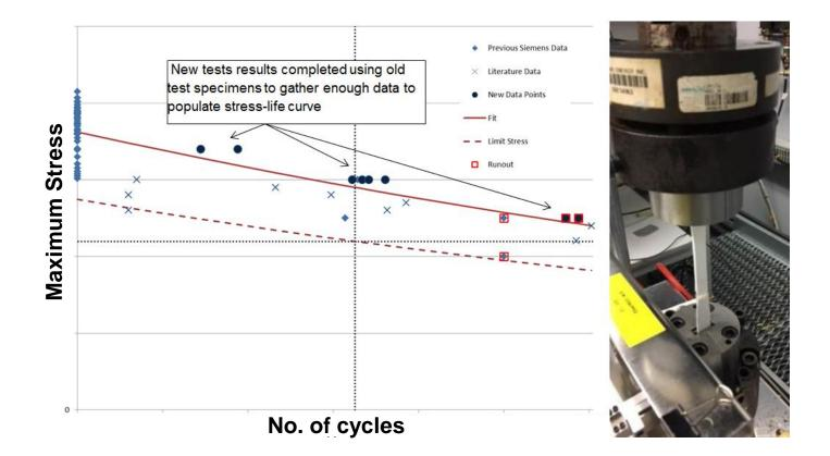
Comparison of current CMC to ca 2005 database shows good agreement (Lower cost 3000 denier fabric used in current design) Testing of involute layup specimens in progress
