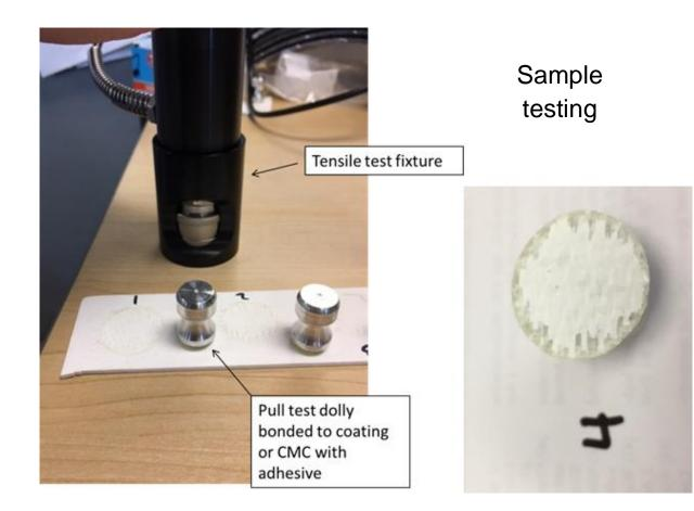
CMC-TBC bond test : 1-day procedure established at CLAB
