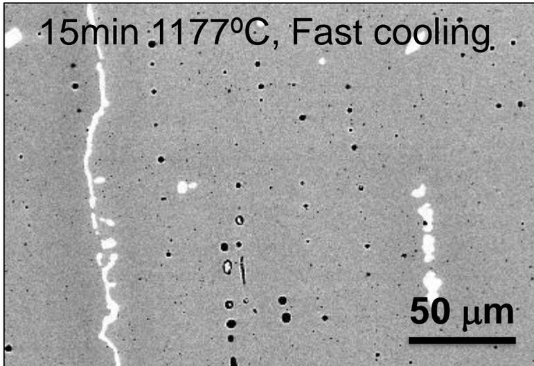
Main microstructure differences between as fab, annealed and HIP'ed HX are voids and precipitates in the grains
