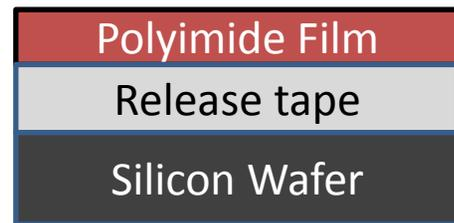
**1. Adhere Polyimide to Silicon wafer and prepare surface**
