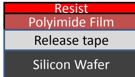
**2. Spin coat a chemical resist to the surface**
