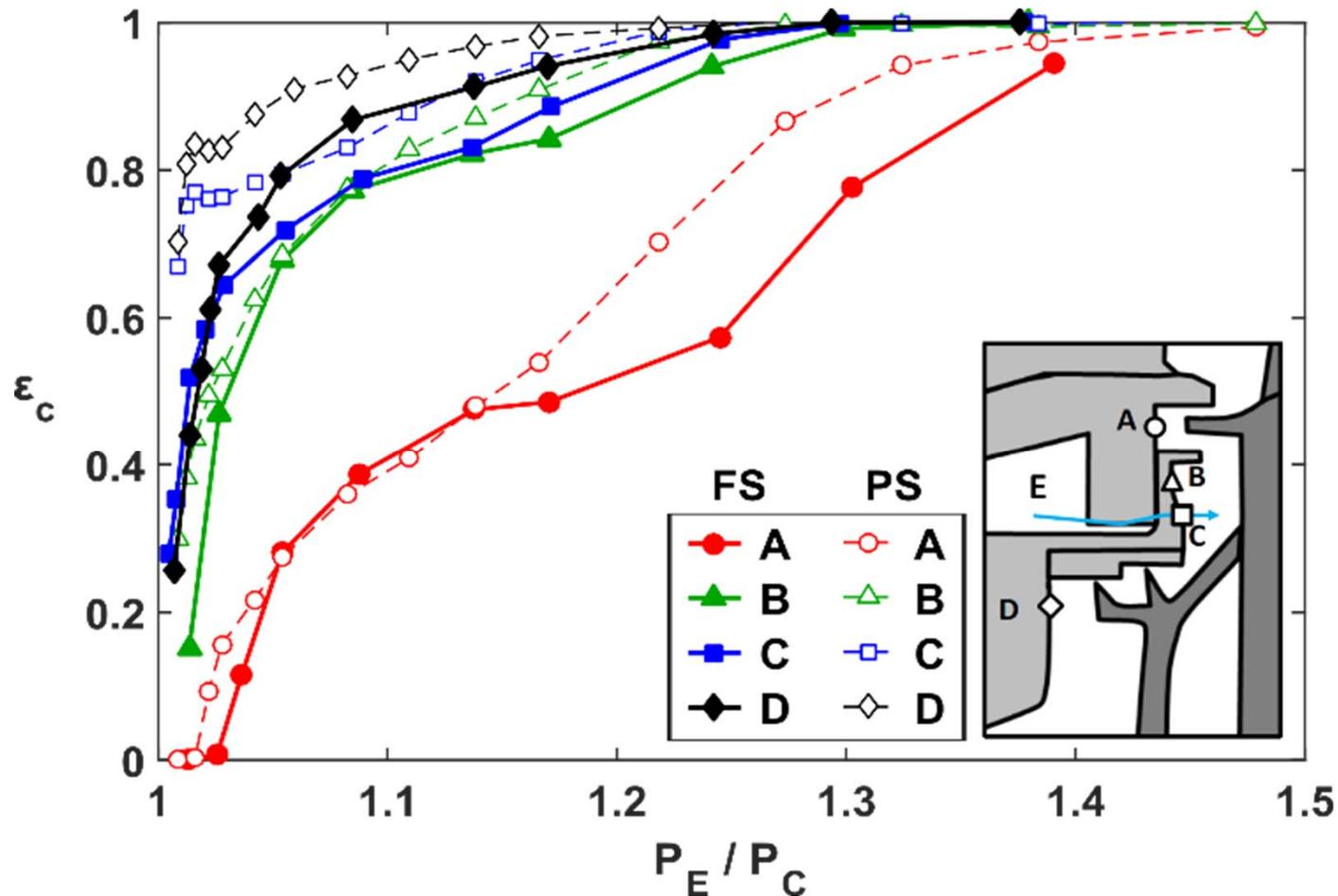
Inflection point in the data was detected in sealing effectiveness, which occurred when rim seal and rim cavity pressures agreed
