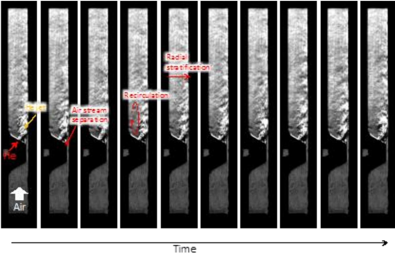
**Stratified Flow from Rapid Expansion Leads to Recirculation Region and Poor Mixing, Potential for Instabilities**
