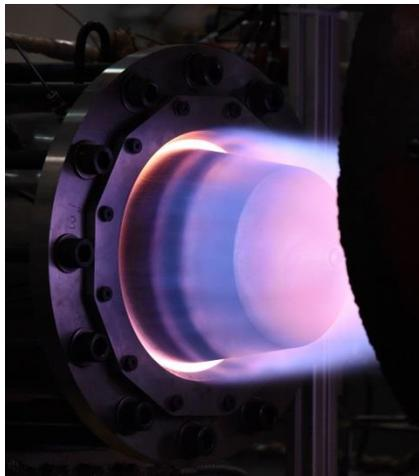
9.4-inch RDE has been delivered to Purdue. First test in November 2017
