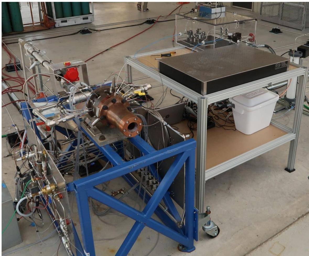
**SwRI Test Stand with RDE/Diffuser Assembly and TDLAS Equipment**
