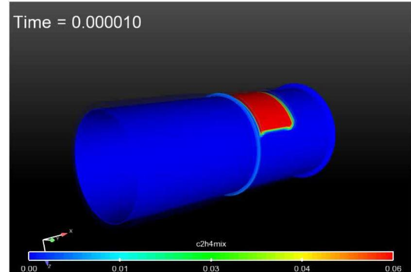
**Quasiglobal Kinetics with Special Treatment of Source Term to Capture Detonation Waves**
