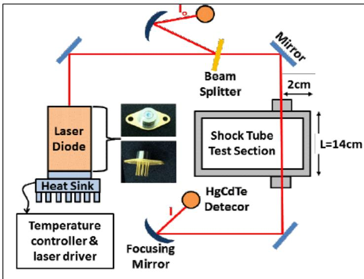
UCF setup for high-speed unsteady measurements of pressure, temperature, species, density and axial/tangential velocities
