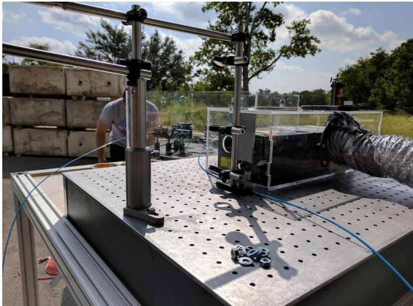
**UCF's TDLAS and PIV Laser Installation at SwRI (RDE/Diffuser to left of picture)**
