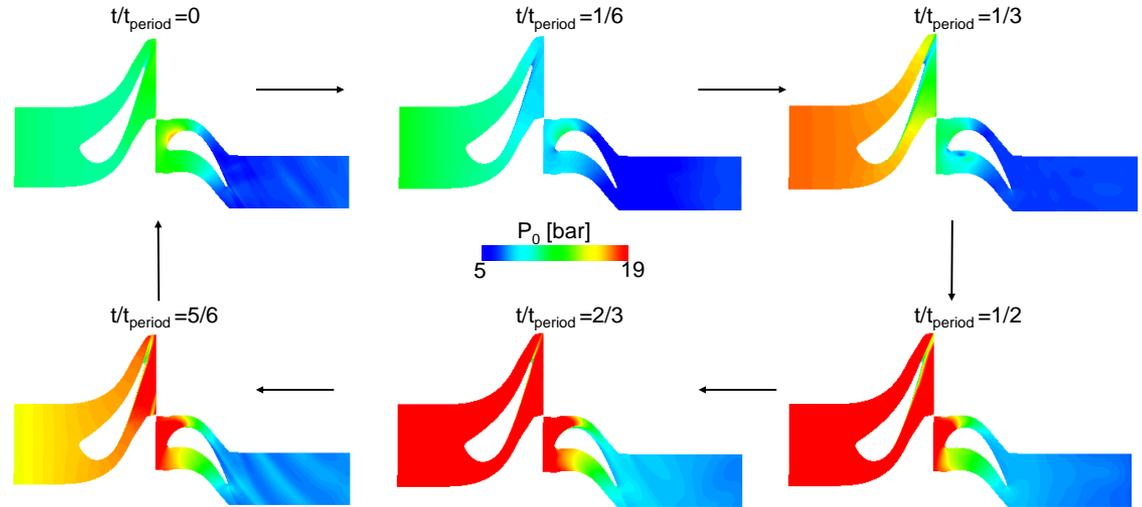
One periodic cycle of an URANS stage simulation (Mach=0.3,  $f=1$  kHz, and  $A=37.5\%$ )
