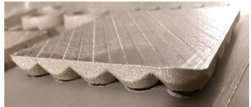
Failed using generic support design
