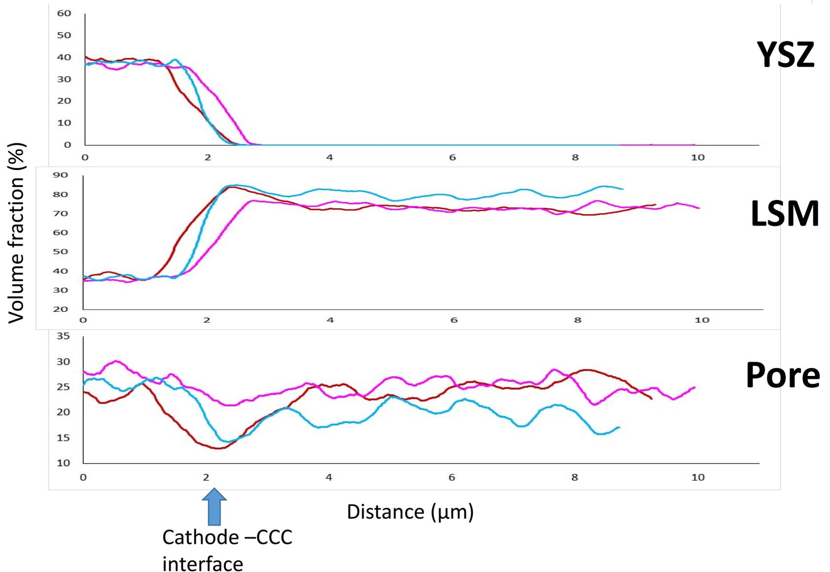
In LSM 85-90 (A) and LSM 80-98 (C), at cathode-CCC interface:
