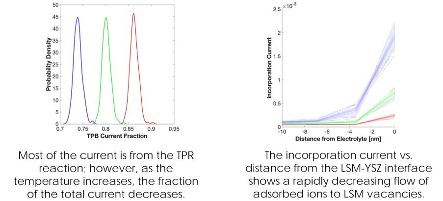
Most of the current is from the TPR reaction; however, as the temperature increases, the fraction of the total current decreases.
