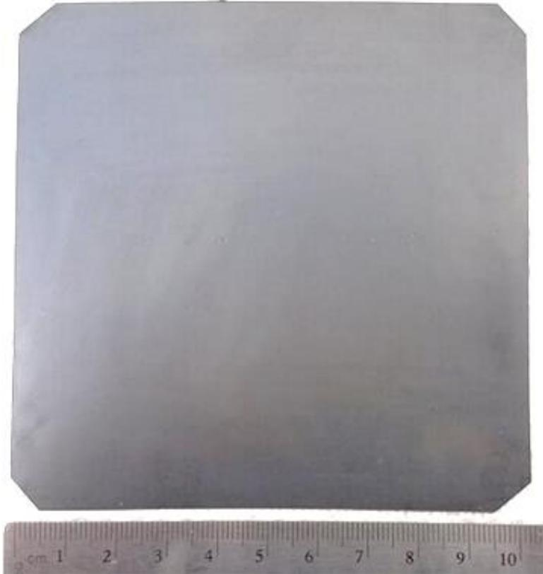
50% fracture strength of Gen. 1 (Ni-cermet) half-cells (4 pt. bend)
