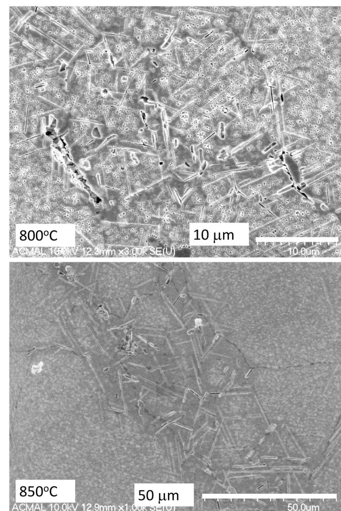
Fig. 3.  $\eta$  phase (needles) formed in Nimonic 263 after 1,000 hours at 800°C and 850°C.
