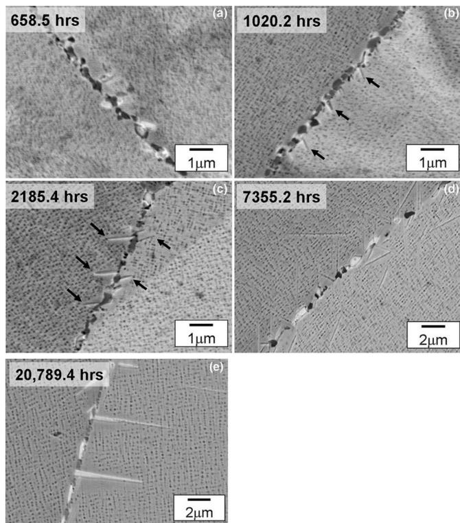
Fig. 1. Evolution of  $\eta$  phase precipitates (needle shape) at grain boundaries in Alloy IN740 exposed at 750°C. Shingledecker and Pharr, 2012.
