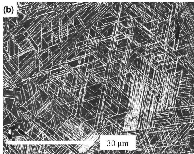
Fig. 2. SEM micrograph of an alloy based on Nimonic 263 containing only  $\eta$  phase in a Widmanstätten plate microstructure. Wong et al., 2015.
