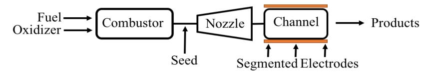
• Early and more recent MHD research has focused on subsonic MHD flows of oxy-enriched preheated air and pulverized coal combustion
