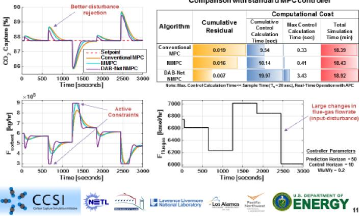
Controller responses to drastic plant-load changes – Comparison with standard MPC controller
