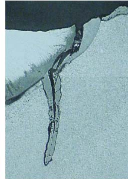
Superheater tube attachment fatigue cracking
