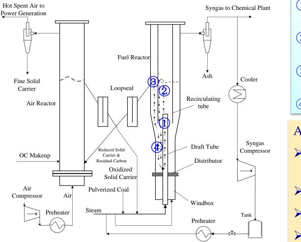
Draft tube (>1000 °C) fast pyrolysis, eliminate tar
