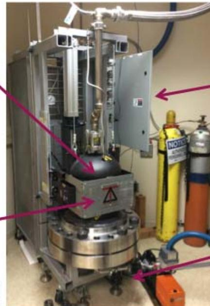
Deltech DT-29-PV-66 controlled pressure high temperature furnace
