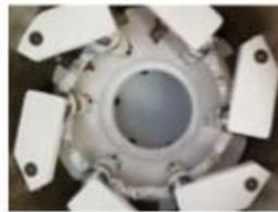
furnace interior with SiC heating elements
