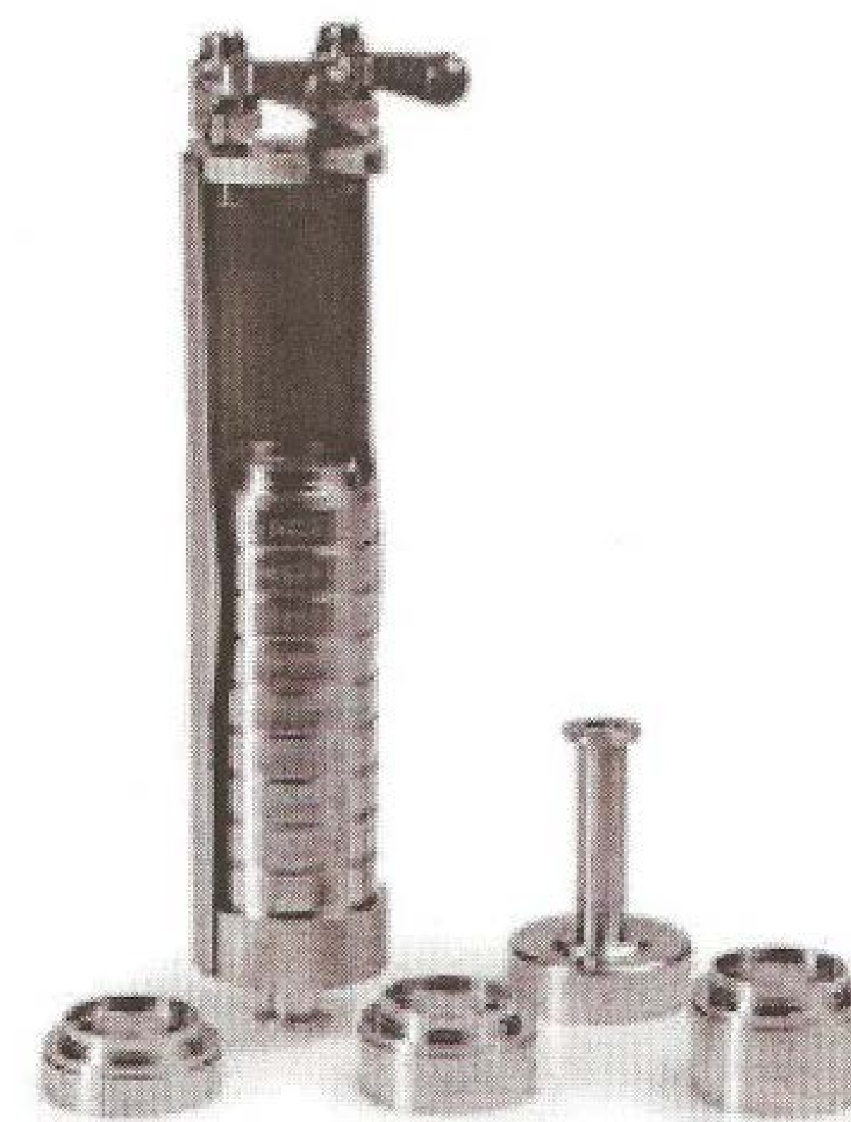
13 Stage DLPI showing aerodynamic cut-points for each stage
