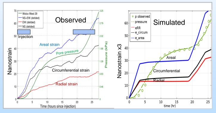
Characterizing and Interpreting the In Situ Strain Tensor During CO<sub>2</sub> injection Aug 2, 2017 NETL Carbon Storage Review
