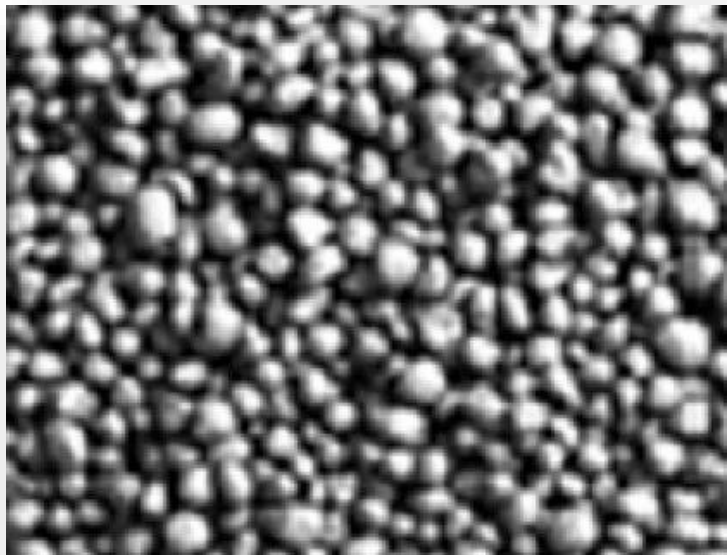
Typical ceramic proppant 20/40
