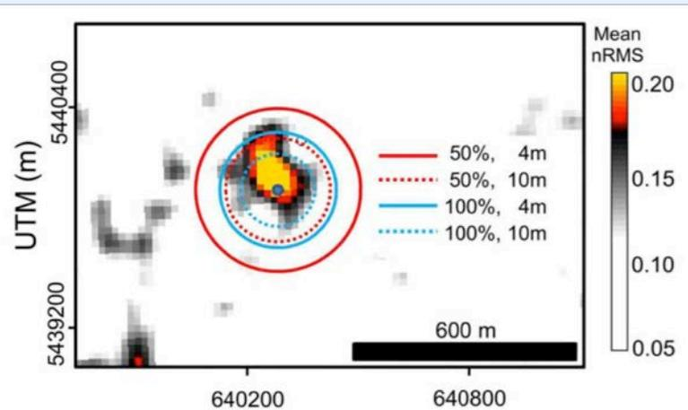
Enlarged portion of the post-injection nRMS map for the upper Deadwood interval. Superposed are circles representing the area of a hypothetical cylindrical CO<sub>2</sub> plume for assumed CO<sub>2</sub> saturation (50% and 100%) and thickness (4 or 10m) within this zone.
