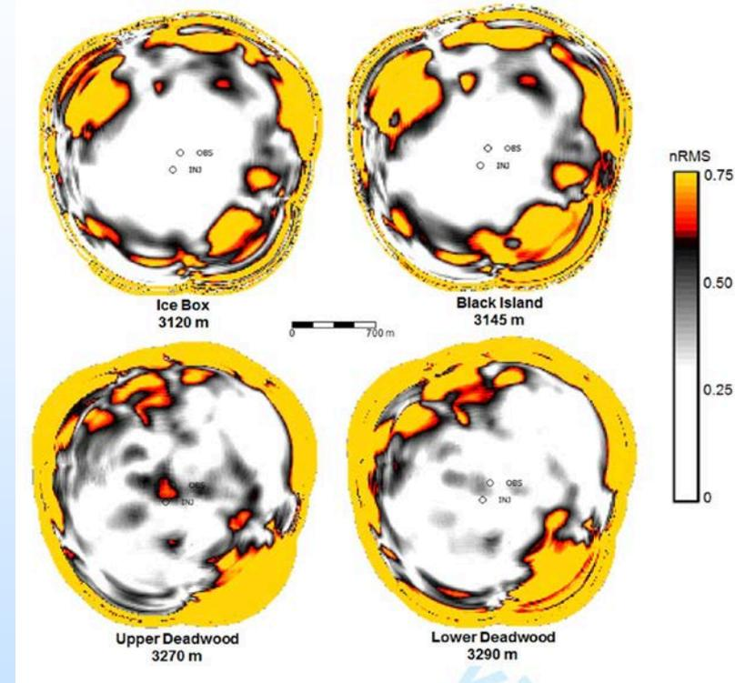
Plan view of nRMS difference images for the reservoir caprock (Ice Box formation and 3 intervals where CO<sub>2</sub> is injected). nRMS values within a 20 m thick window
