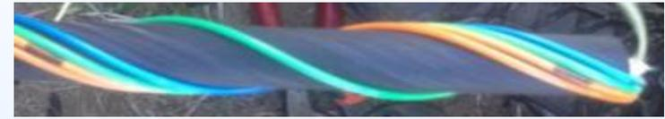
HWC cable: 30-deg winding, single SMF fibre
