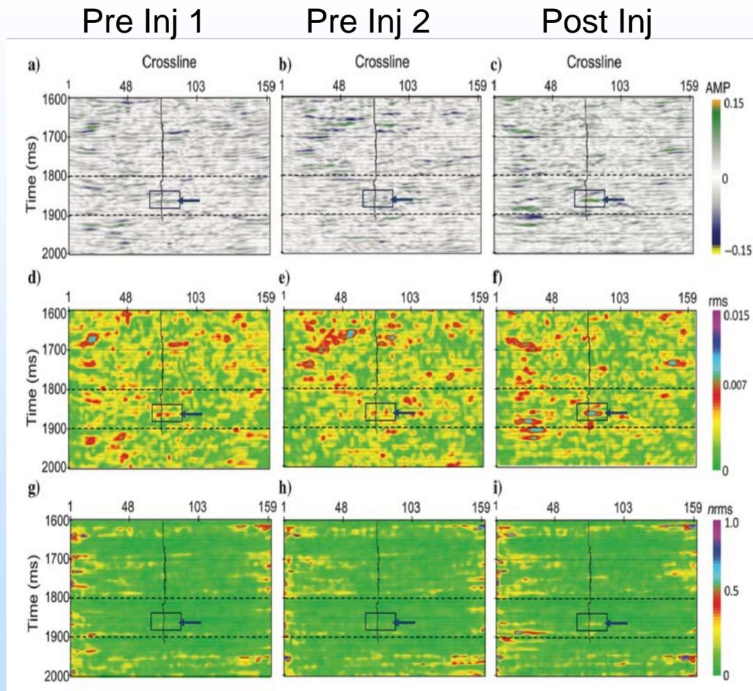
Difference of monitor surveys relative to baseline: Amplitude difference for (a) monitor 1, (b) monitor 2, and (c) monitor 3. The rms amplitude difference for (d) monitor 1, (e) monitor 2, and (f) monitor 3. The nrms amplitude difference for (g) monitor 1, (h) monitor 2, and (i) monitor 3. Superposed is the  $V_p$  log. The reservoir is demarked by the dashed black lines.
