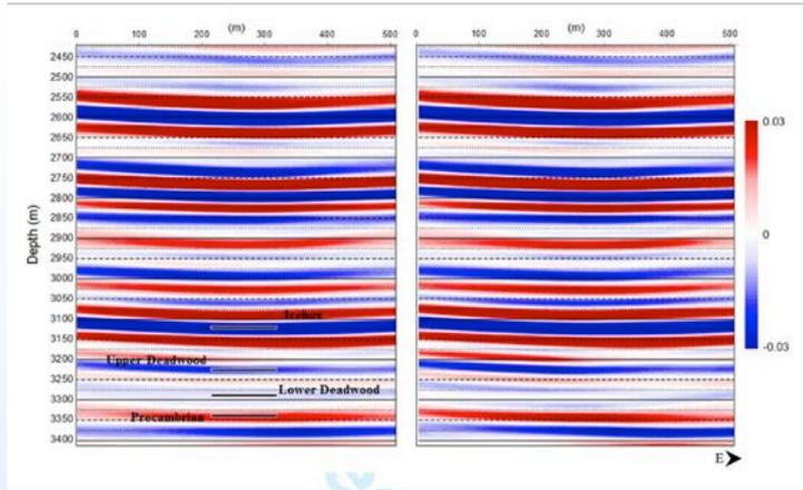
**nRMS of monitor-baseline differences** for a 75 m window in cross-sections through observation (left) and injection (right) wells. In both difference sections, a nRMS  $\approx$  0.9 anomaly is present at a depth of  $\sim$ 3275 m (in dashed circle).
