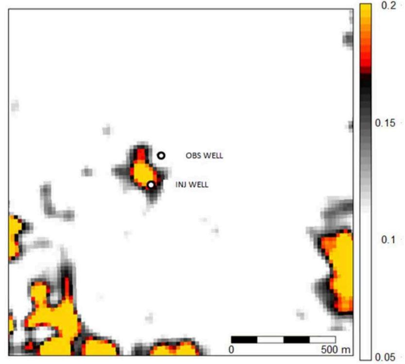
Plan view of nRMS difference images in the upper Deadwood showing VSP result (left) and surface-based result (right).
