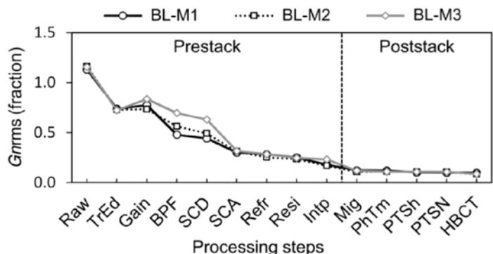
The Grms computed within the window 700–2000 ms on stacked traces for post- and pre-CO<sub>2</sub>-injection data sets.
