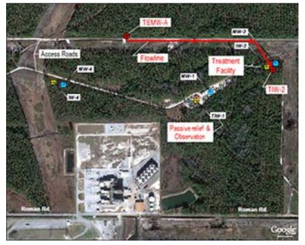
BEST project infrastructure layout showing the proposed location of the extraction well (TEMW-A), injection well (TIW-2) and flowline, and the existing passive-relief well (TIW-1)
