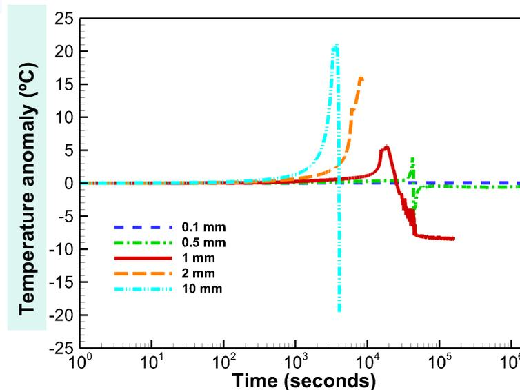
The temperature signal is very weak when the aperture is below 1 mm (< 1 °C) due to very small leakage rate.
