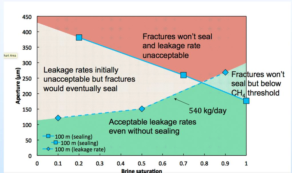
Developing a New ROM that incorporates impact of chemistry and mechanical alteration 11
