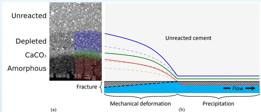
Damage zones of concern for a 10 MPa overpressure
