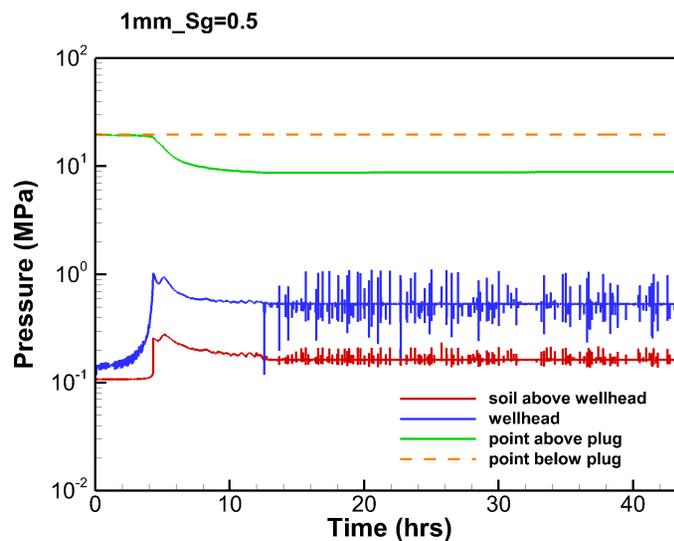
Temporal patterns of P, T, and gas saturation may provide detectable signatures of low-flow-rate leakage in shallow subsurface around abandoned well
