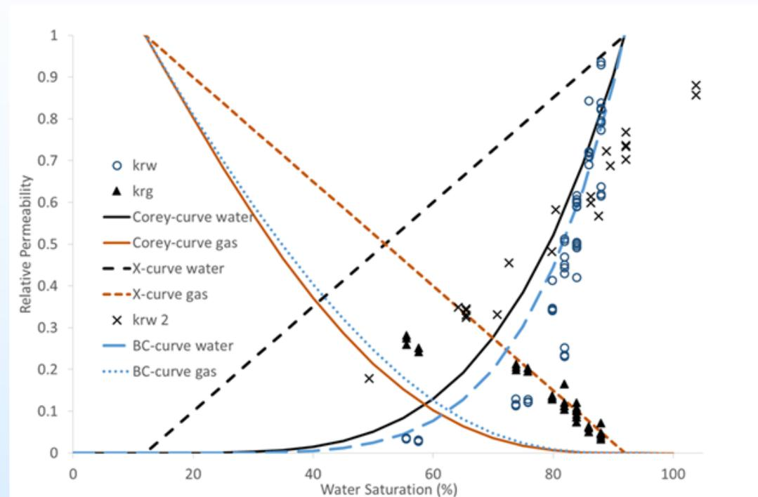
Cement fracture aperture size and complexity influences which relative permeability model is most valid
