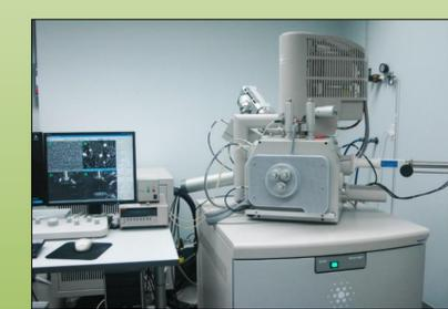
Scanning Electron Microscope used for feature relocation before and after dry/wet CO<sub>2</sub> exposure.
