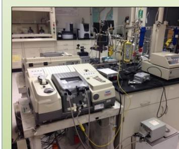
Left. FT-IR Spectrometer used to conduct In-situ high temperature and pressure experiments.
