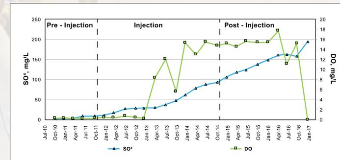
Figure 2. Monitoring data influenced by a leaky sampling pump in well G102.
