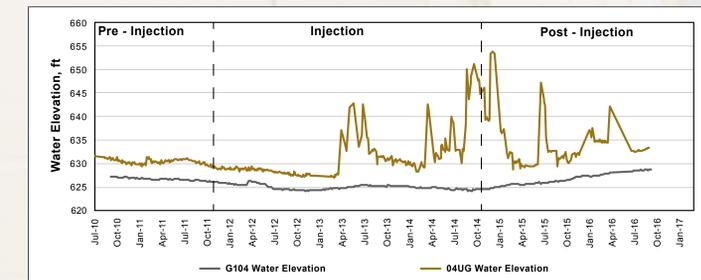
Figure 5. Groundwater elevation in G104 and 04UG. Higher differential elevation in 04UG potentially causes downward flow from Glasford (04UG) to Pennsylvanian (G104) aquifer.
