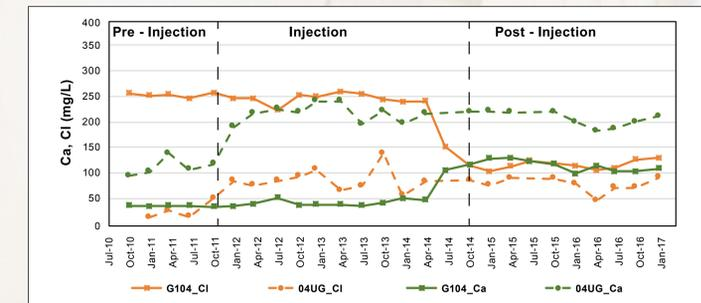
Figure 4. Calcium and chloride concentrations in wells G104 and 04UG.
