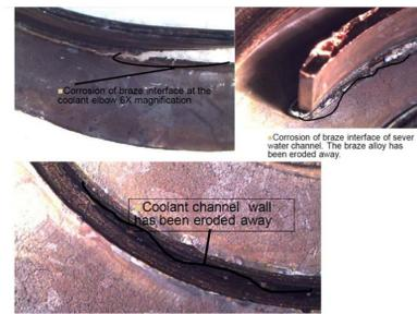
**Need:** Isolate metals from coolant fluid (water, ethylene glycol)
