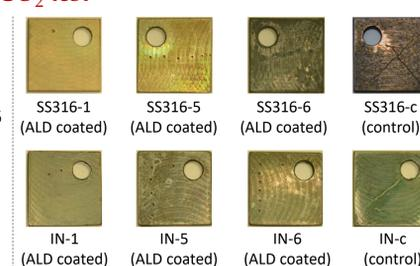
Photographs of ALD coated and control (SS316-c and IN-c) samples after 500 hour exposure in sCO<sub>2</sub> test apparatus
