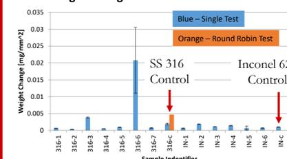
Ceramic coatings were deposited by ALD onto SS316 and Inconel 625 coupons, the weight change was measured after a 500 hour sCO<sub>2</sub> exposure
