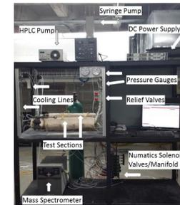
Photograph of the sCO<sub>2</sub> autoclave exposure facility at the University of Wisconsin
