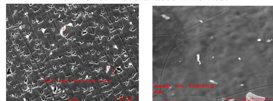
Uncoated sample - heavily pitted      Coated sample - no pitting
