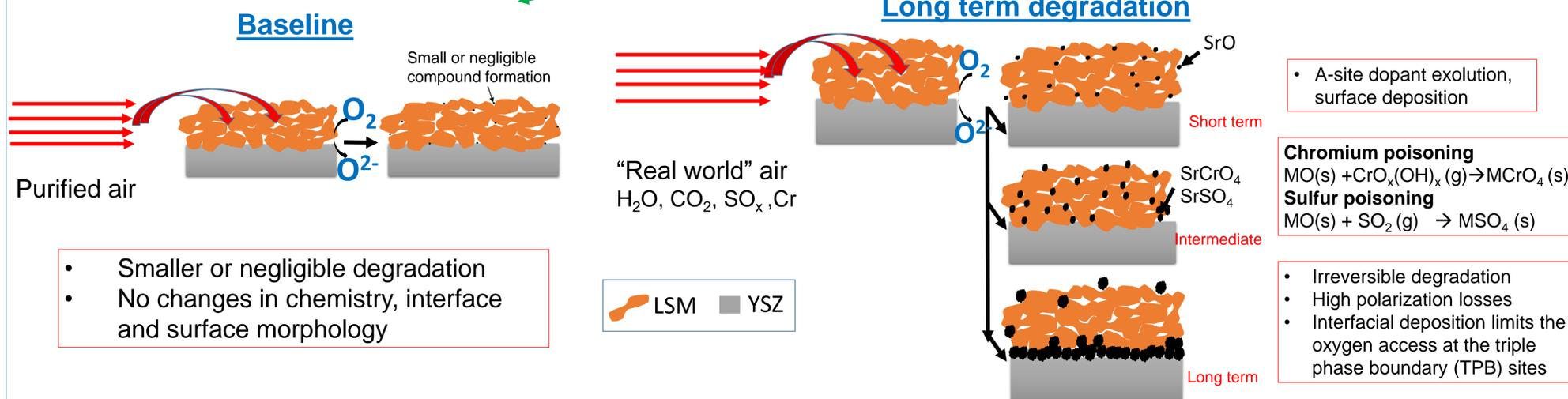
**Baseline:** Negligible degradation of SOFC electrochemical cell under purified air, **Chronological degradation:** Different stages of degradation occurring over time in an electrochemical cell under the "real world" air containing both extrinsic and intrinsic impurities through surface and interfacial compound formation
