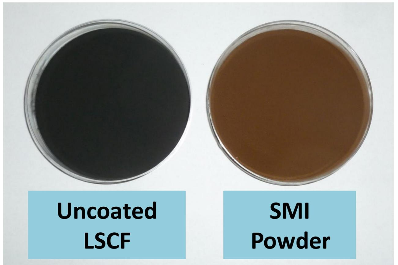
During Phase I, SMI produced several samples of surface functionalized LSCF powder. The typical batch size was 20 to 25 grams in Phase I. This can easily be scaled to larger batch sizes in the future. The primary variable investigated in Phase I was the total amount of surface material applied, expressed in moles per kg of LSCF base powder.
