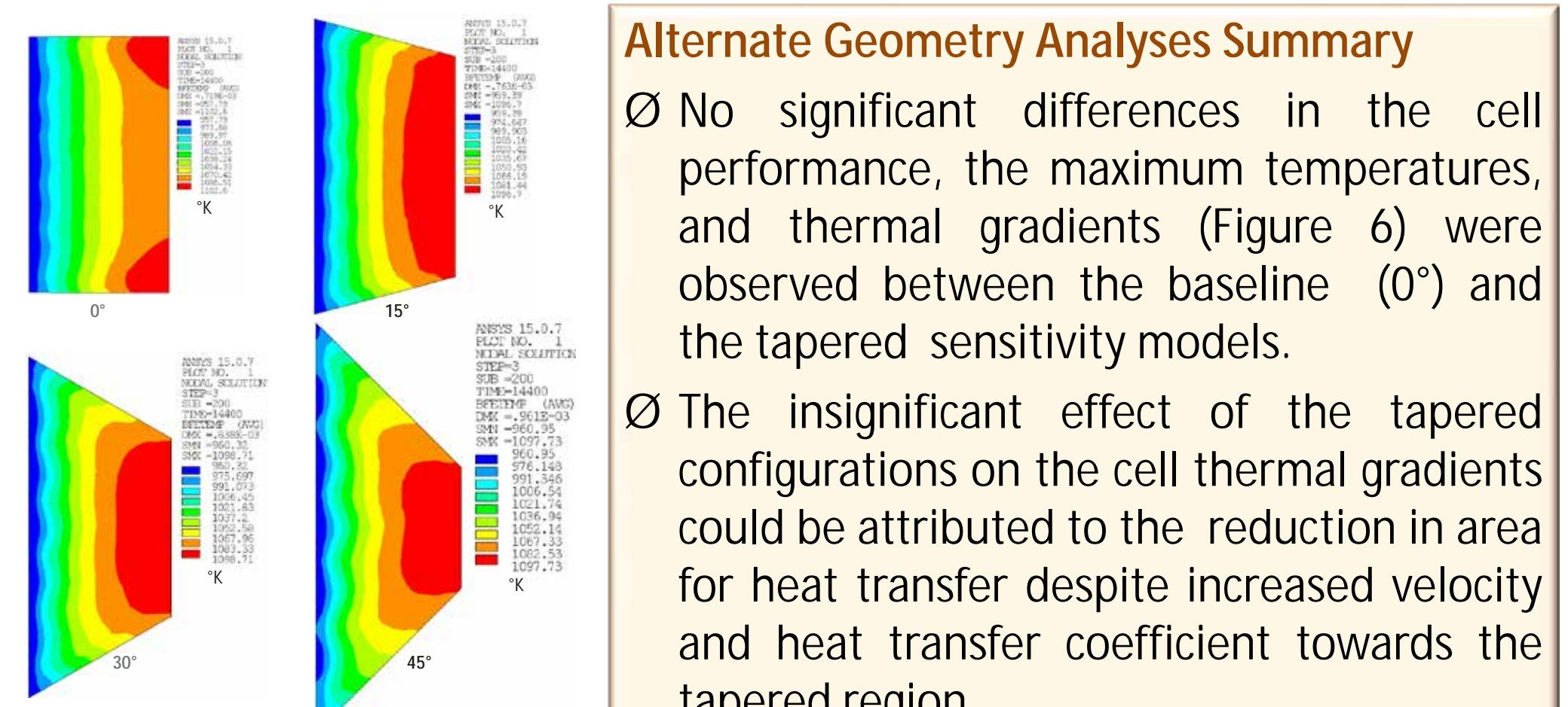
Figure 6: PEN operating thermal gradients from the baseline, 15°, 30° and 45° models
