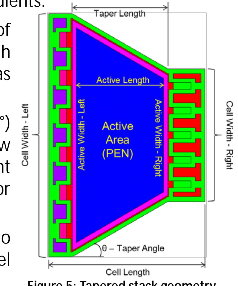
Figure 5: Tapered stack geometry
