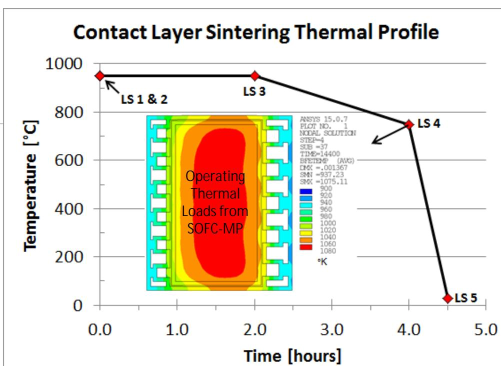
Figure 3: Thermal profile & load steps in contact layer sintering and stack reliability FEA simulations
