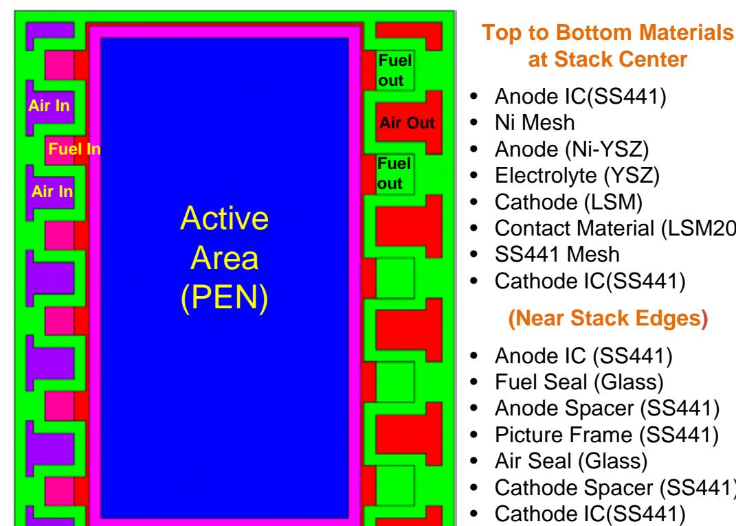
Figure 2: Baseline FEA configuration for cathode contact layer and stack reliability evaluations
