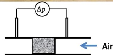
Pressure drop measurement setup
