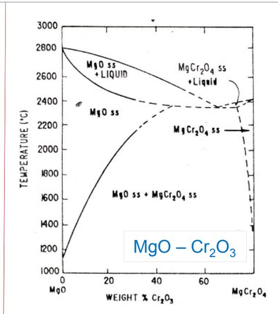
Oxide solid solutions and mixtures from Alkaline earth and Transition metal group are preferred and considered over single phases due to chemical stability and resistance to interactions with gas phase impurities.
