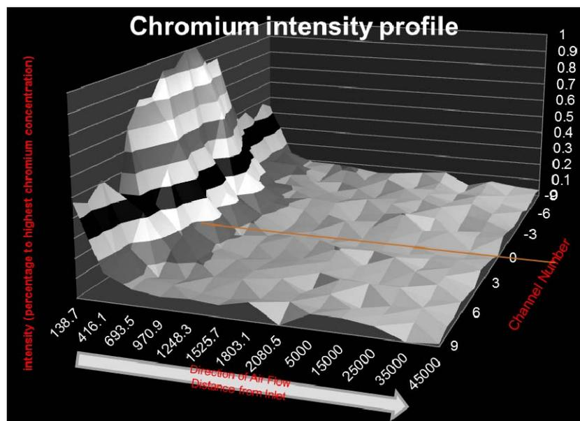
Higher Cr intensity (analysis performed using EDS technique) is observed near the air inlet (~ 1200 micron). Flat Cr profile is observed over the entire length after ~1500 micron indicating little/no Cr.
