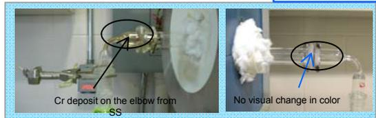
Significant reduction in Cr evaporation has been achieved by alloy, atmosphere and materials chemistry modifications.
