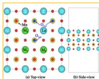
Top-view and side-view of the (La,M)O terminated (M = Ca, Sr and Ba) model with the all-possible dopant substitution
