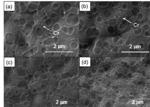
SEM micrographs of the YSZ electrolyte surface in contact with a LSM electrode coating in the presence of a FeCr alloy at 900 C after cathodic polarization for (a) 5 min, (b) 15 min, (c) 30 min, (d) 4 h,
