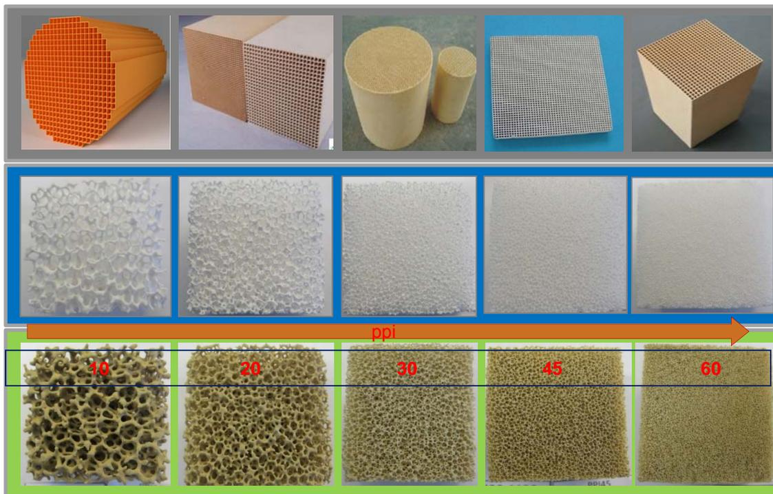
A wide variety of support materials and configurations are available for application in SOFC system. Selection will be based on:
