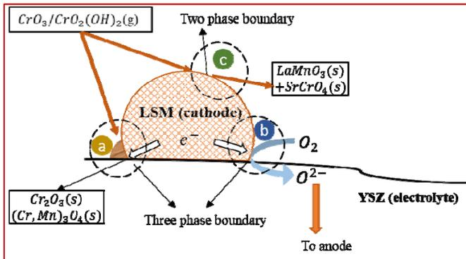
Schematic of chromium poisoning at three phase boundary (a and b: Three phase boundary reactions; c: Two phase boundary reaction) (TMS Meeting, Feb. 2016)
