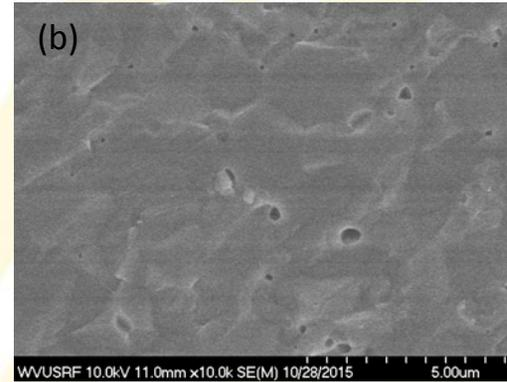
Microstructure of GDC pellets (a) sintering at 1450 without sintering aid and (b) sintering at 1300 with 2mol% iron oxide
