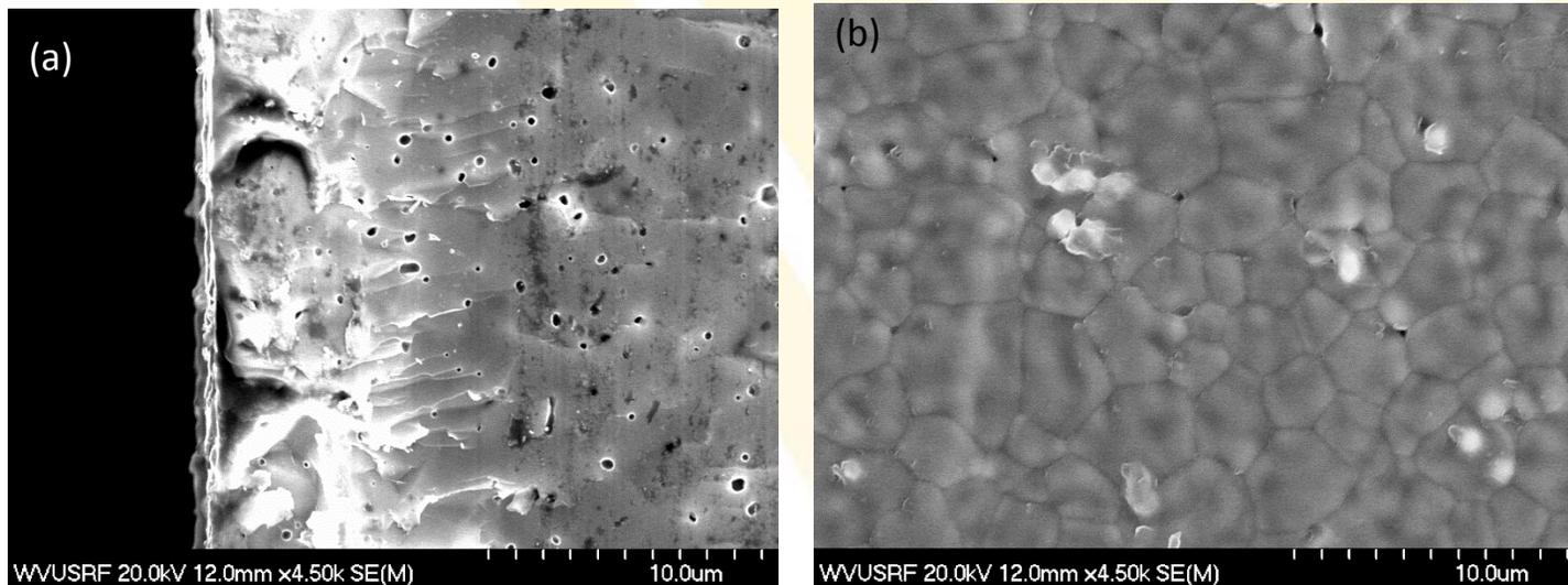
(a) cross - section and (b) microstructure of polypyrrole coated on YSZ before sintering
