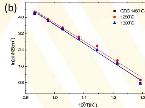
(a) temperature dependence and (b) Arrhenius plots of the ion conductivity for GDC with and without 2mol% iron oxide after sintering at 1300°C for 4h
