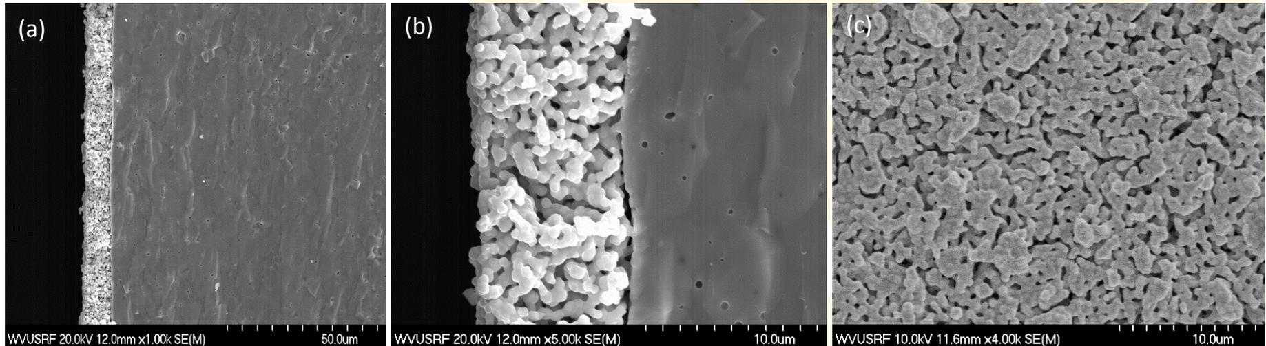
Morphology of GDC deposited on the polypyrrole coated YSZ pellet after sintering at 1300C
