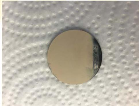
Macrostructure of deposited GDC before sintering
