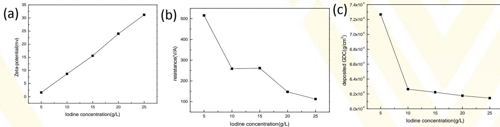
Effect of iodine concentration on (a) Zeta-potential, (b) suspension resistance and (c) the amount of deposited GDC
