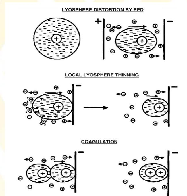
Schematic representation of electrical double layer distortion and thinning mechanism
