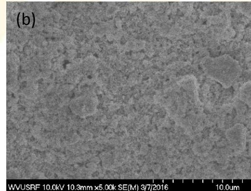
(a)cross-section and (b) surface morphology of GDC layer before sintering
