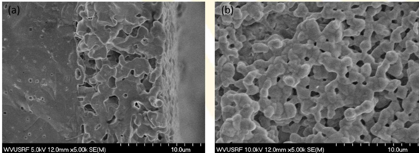
Morphology of GDC with sintering aid deposited on the polypyrrole coated YSZ pellet after sintering at 1300°C
