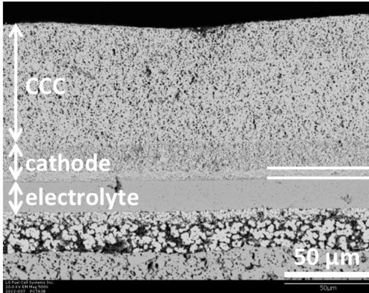
Densified layer (between two white lines) is ~5 μm thick (SEM image, courtesy of LGFCS)
