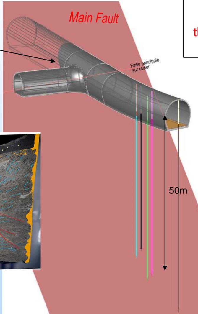
The unaltered structure of the Main Fault has been accessed through gallery outcrops and fully cored boreholes
