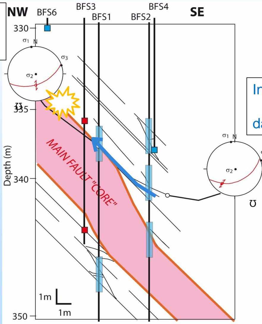
Injection N°2 in the fault damage zone
