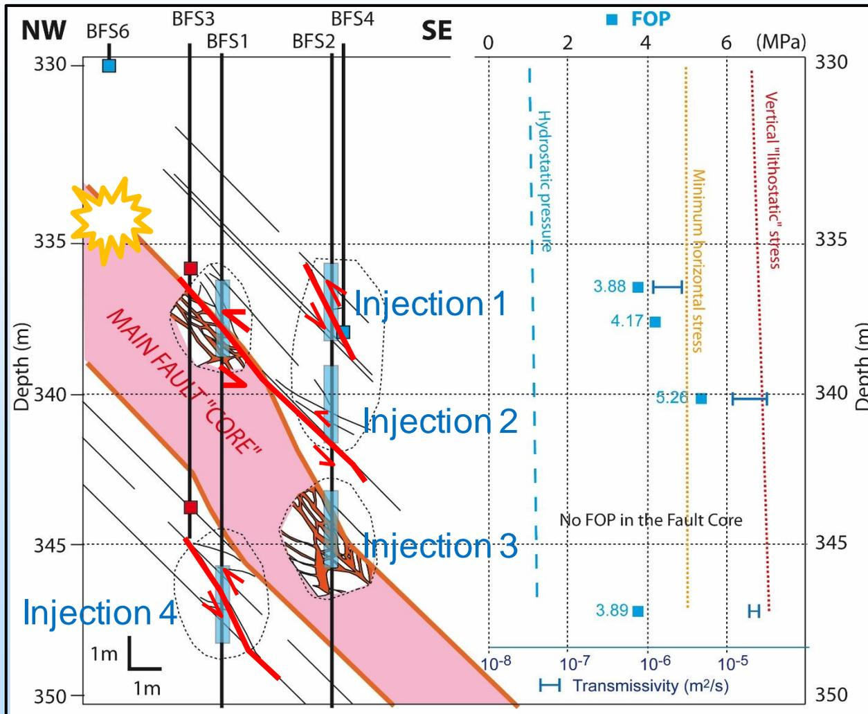
Fault planes reactivated during the different injection tests
