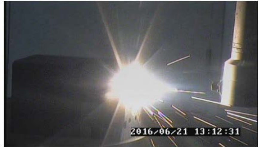
Laser Firing 3kW on Sample (4.2 kW cm -2 )
