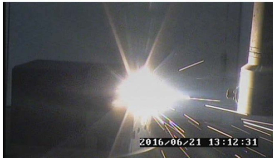
Laser Firing 3kW on Sample
