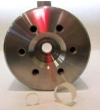
Hydrostatic cell for study of pore and saturation evolution under uniform pressure conditions (300 MPa, 43,500 psi; 200  $^{\circ}\text{C}$ )
